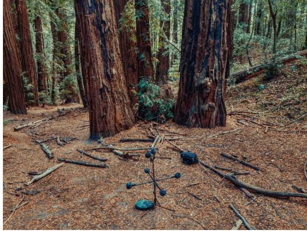
Beverly's 4.0.2 set-up with MKH 8020 and MKH 8040 on the forest floor
