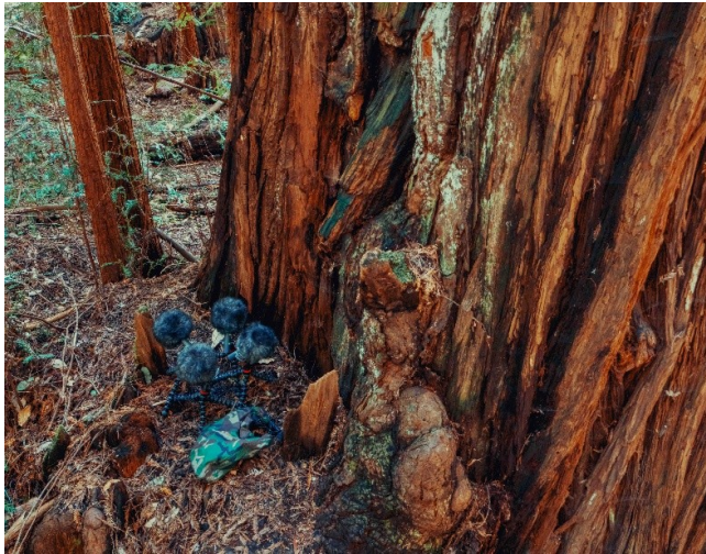
Four MKH 8040 in a double ORTF configuration at the base of a redwood tree. The mics recorded the outward sounds, while contact mics clipped to the bark recorded the internal sounds of the tree
